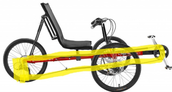
Figure 1: Example of Recumbent Tricycle with Rear Wheel Driven Drivetrain ( https://www.basicallybicycles.com/product/sun-seeker-eco-tad-sx-1694.htm )
