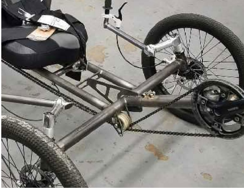
Figure 15: Zoomed Image of Front Set of Skateboard Wheel Idlers on HPV Drivetrain
